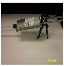
To assemble, hold tubes with tip facing upward. First, remove protective cap from tube set. Next, remove the two end caps from each tube. Place the control valve onto the end of the tube and place the static mix nozzle over the tube set ends. Finally, slip the screw collar over the tip and tighten on the tube set and then place the tube set into the tube applicator.
